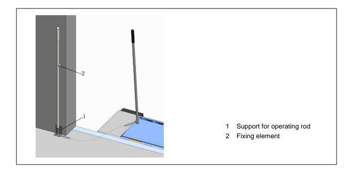
A wall thickness of B < 240 mm requires two additional support elements and a console.
